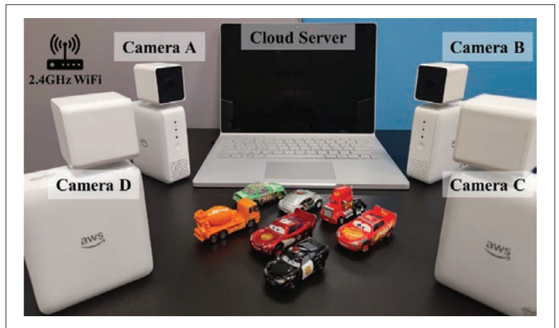
FIGURE 4. A FEVA-supported multi-view vehicles 3D reconstruction system implementation.
